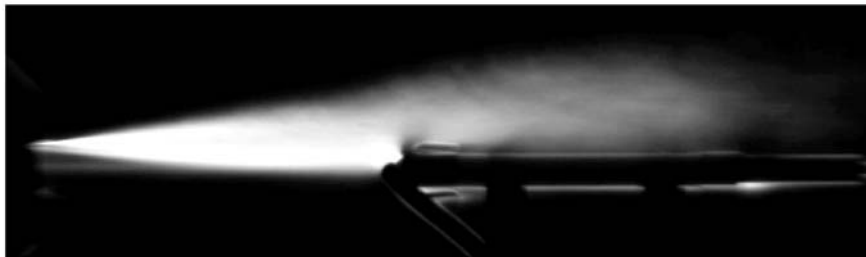
Fig. 2. Shadow pattern of the process of blow-over of a flat plate by a two-dimensional air jet.
